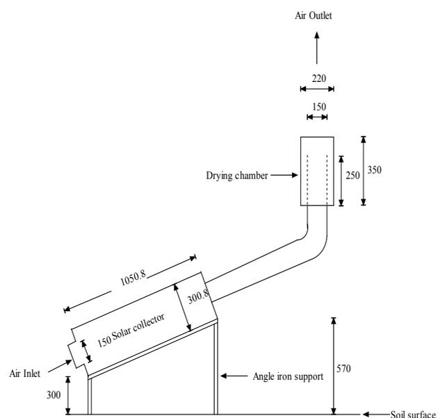
Figure 1. Schematic view of the experimental solar dryer setup (all dimensions in mm)
