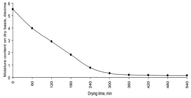
Figure 3. Drying curve of moisture content versus drying time of whole okra pods during the first day of the drying process
