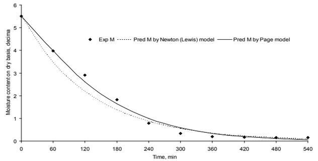
Figure 4. Experimental and predicted moisture contents of whole okra pods during the first day of the drying process
